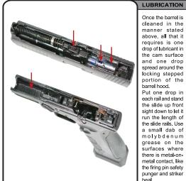
ocking stepped portion of the parrel hood. Put one drop in the slide up front sight down to let it run the length of the slide rails. Use a small dab of molybdenum grease on the surfaces where there is metal-on-metal contact, like the firing pin safety punger and striker heal.
